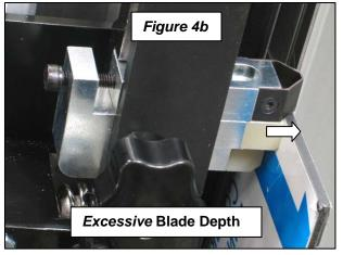
**Tip:** As a general rule, allow a minimum of 0.5mm (1/64"+) of the material's plastic core, plus the aluminum skin, to remain after the groove has been cut. Cutting too deeply may compromise the strength of the material when bending afterwards.
