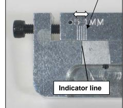
Raise the FSC cutting head above the top edge of the sample sheet of material, and tighten the head locking knob to keep it in place. Insert the Vgroove tool into the FSC cutting head, as shown, and tighten the tool locking knob (Figure 3).
