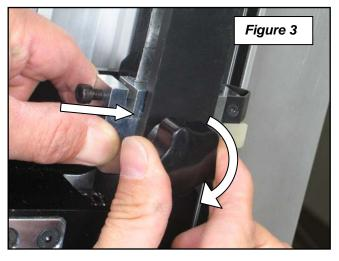
4. Loosen the head locking knob, and slowly lower the head so that the V-groove blade is resting on the top edge of the sheet of material. Visually check the front edge of the blade, and see how far into the material's thickness it extends (Figures 4a and 4b below). Depending on the amount of material you wish to remove, it may be necessary to adjust the blade depth again. Make a test cut in the composite to verify (see next section below).
